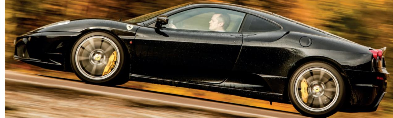
vented bonnet, strakes in the sills, a loftier tail spoiler, forged wheels and bumpers featuring movable flaps that reduced drag at speed. The engine, meanwhile, received a power hike to 597bhp. This new strain weighed 90kg (198lb) less than the car that bore it, and was reputedly good for 0-125mph in a blistering 9.1 secs.
