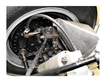
brakes have been fitted with huge aluminium air scoops which appear to be of great age. In all probability these were fitted in the early days of its life in the USA. The back plates have been drilled for improved air circulation in a typical 1950's USA style. The brake linings remain the old USA linings, which still show plenty of thickness.
