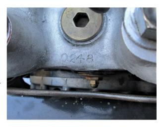
The sump pan is the correct two-part cast aluminium type. It has a flattened pan shape to lower the overall height of the engine. It has cooling fins running the full length of the underside, as the production C type was not equipped with an oil cooler.
