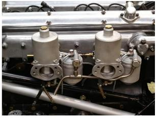
overhauled in the USA. Because of these factors, it was decided to leave the engine and cams "as is". The drivability has not suffered and although the bottom end torque is slightly reduced, the trade-off is that the performance is actually now very good. The cam covers and sump were removed to check the internal state of the engine and the bearings, which we confirmed were in good condition, as we had hoped.
