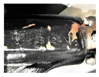
use or tours. The original 3.54:1 ratio has therefore been sourced and fitted on an exchange basis. Interestingly the speedometer now reads correctly again!
