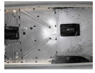
Original photographs of the car when new, show that strangely it was never fitted with the normal tubular bonnet stay, listed as a standard part (BD6403) for all C types. A cable stay will not work in windy conditions as we quickly discovered. Consequently one has now been made and fitted exactly to pattern.
