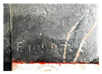
The second engine number appears on the cylinder head, stamped on the vertical front face of the "vee" between the camshafts. Reassuringly, it is also stamped into the raw cast surface with no sign of grinding.
