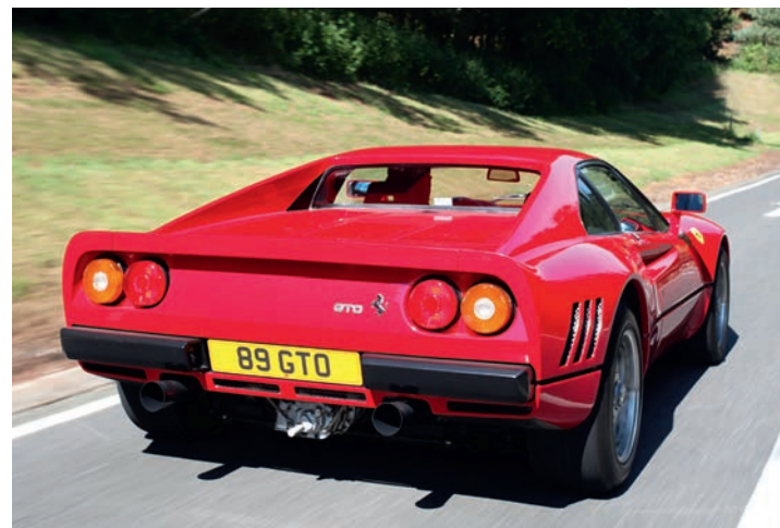
Below: Michelotto twin trumpets were a factory option in place of quad pipes; steering is meaty but wonderfully precise; five-spoke Speedline rims
