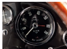
Redline is 6000, but 5000rpm more is safe; recessed fuel cap
