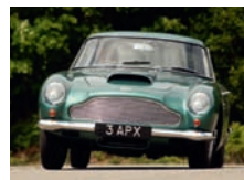
No overriders for GT; shorter doors and no windowframes
