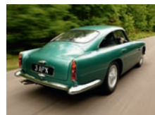
No overriders for GT; shorter doors and no windowframes
