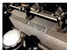
Beautifully finished engine bay; air scoop feeds Weber trio
